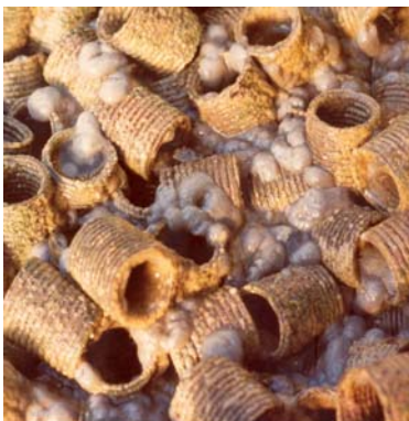
Figure 1. Subbaromyces splendens can form surface growth when media is continuously loaded with wastewater, although growths are normally restricted to lower depths.
