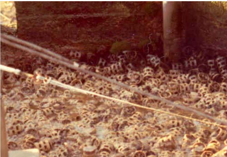
Figure 2. All plastic media types are affected by the fungus, including both random and modular forms.
